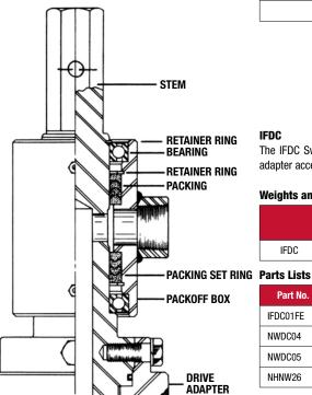
The IFDC Swivel is designed for wet augering or grouting without moving the rig. A semi-finished, bolt-on adapter accepts drive caps 4 1/4" through 6 1/2".
